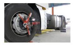
computerised system can now include all data relating to truck wheel alignment, so that technicians can get a real-time comparison of readings against manufacturers' specifications.
